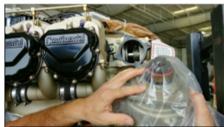
Alternator couples to the engine by gears, not by a belt as in many other light aircraft engines
