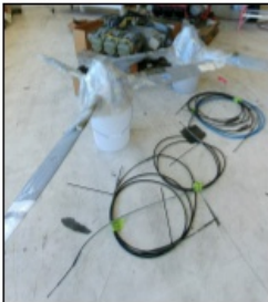
Cables being threaded through the wing between engine & fuselage
