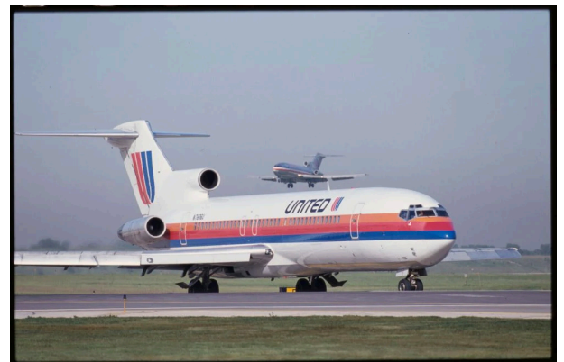
The 727 was the first jetliner to feature an Auxiliary Power Unit (APU). Photo: Getty Images
