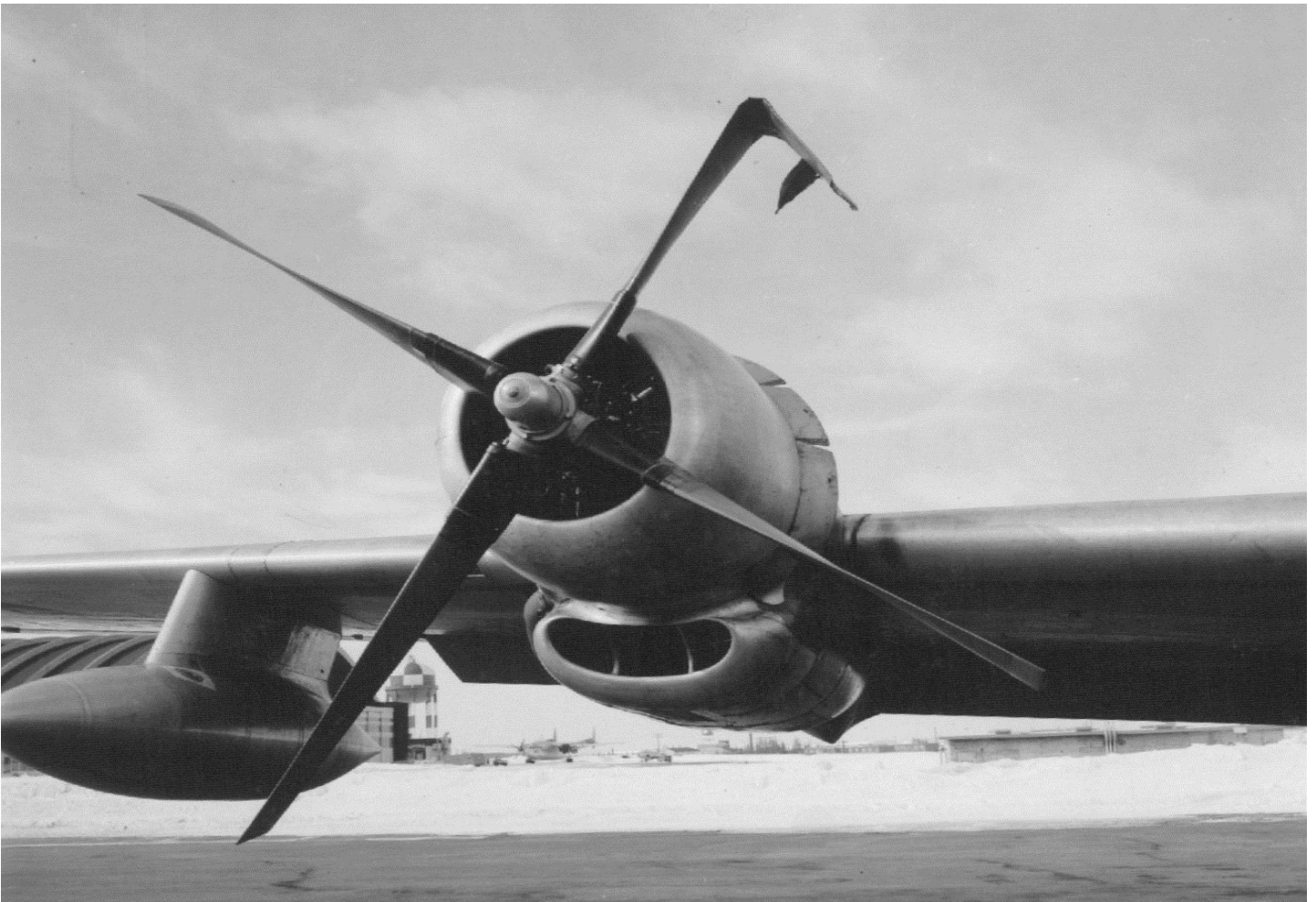
Here is a better view showing how severely the prop blade was bent. If this prop had not been feathered just before the #3 let go, it would have torn the whole engine off the airplane.
